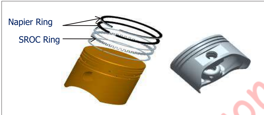
Existing Ring Pack Piston with Ring Assy no:MSP 1/194
